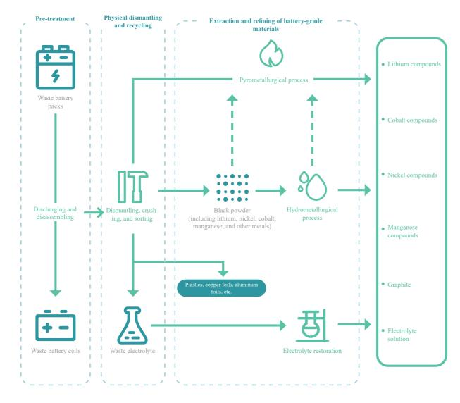
Figure 10. Typical Process for The Recycling of Power Battery Materials (Deloitte, 2022)
