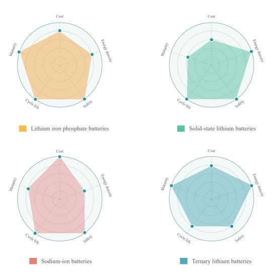
Figure 9. Comparison of Characteristics of Different Types of Power Batteries
