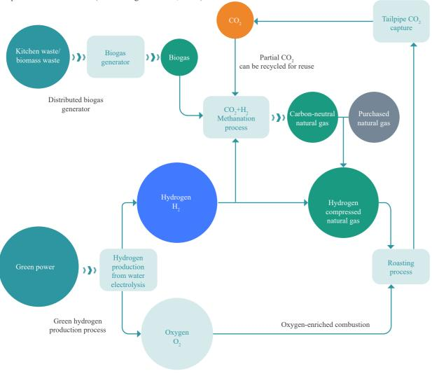
Figure 8. Schematic Diagram of Achieving Net Zero in the Roastinginduced Transformation Process Based on Natural Gas as Fuel
