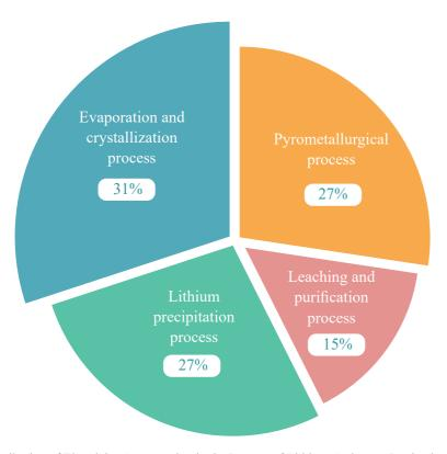
Figure 7. Distribution of Electricity Consumption in the Process of Lithium Carbonate Production Using Sulfuric Acid Roasting Method (Du Guoshan, 2020)
