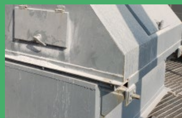
Semi-closed acidification feed beltweighers improved into fully-closed ones
